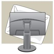
1. After moving the product to face downward, make sure to place it on a soft cloth or a cushion to avoid surface damage.
